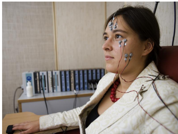
Figure 8: The lab is a.o. equipped with an EMG for measuring facial muscle activities.
